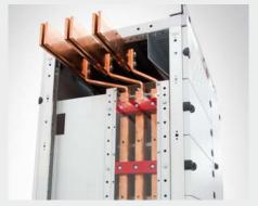
Cabinet - rear busbars with tunnel: cabinet with sections and segregation form 3b. Vertical busbar system placed at the back and horizontal busbar system placed on the top.
