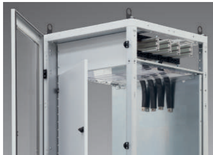
IP55 Attic Power cabinet: structure prepared for the busbar system positioning under the roof of the cabinet, comprehensive of segregations, frontal glass door and sheet inner door.
