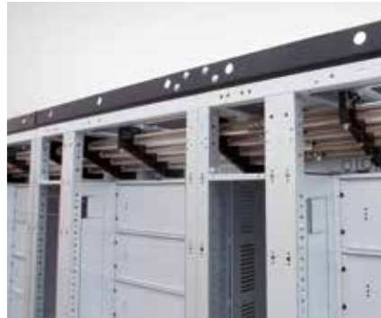
Cabinet - rear busbars with tunnel: cabinet with sections and segregation form 3b. Vertical busbar system placed at the back and horizontal busbar system placed on the top.
