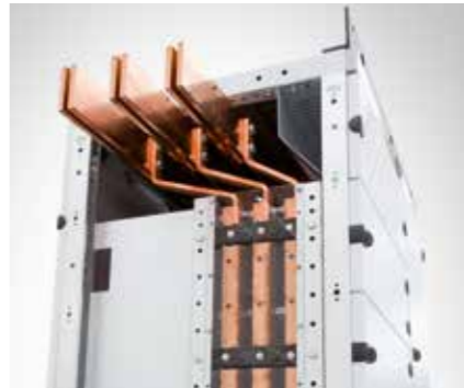
Cabinet - rear busbars: cabinet with sections and segregation form 3b. Vertical and horizontal busbar system placed at the back
