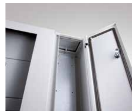
Cabinet with cable housing: Mono-block structure made of welded sheet with a thickness 12/10 mm with cable housing, terminal block or busbar system.
